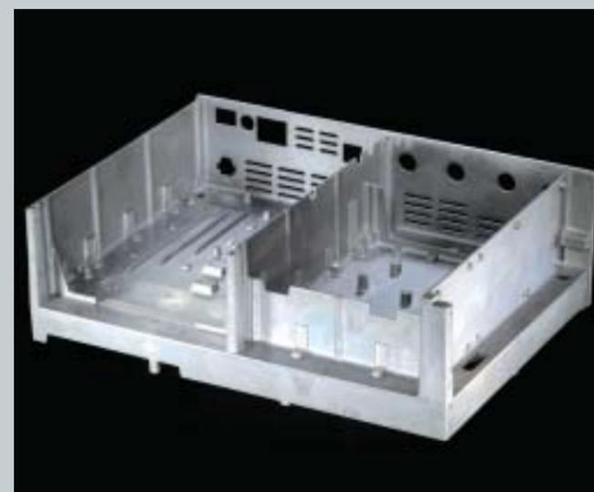
The FT-2000D (200-Watt version) utilized push-pull SD2931 MOS FET devices, operating at 50 Volts, with user-adjustable bias control to ensure the optimum suppression of intermodulation distortion products. The elaborate heat sink design includes a combination of aluminum and 3 mm thick high-conductivity copper plate, with a total heat sink capacity of 2720 cc, ensuring many years of reliable operation of this 200-Watt powerhouse.
