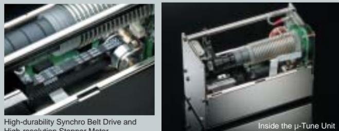
High-durability Synchro Belt Drive and High-resolution Stepper Motor
