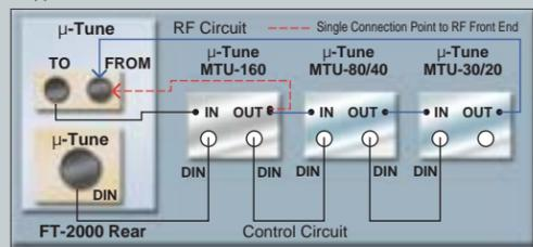
RF  $\mu$ -Tuning Kit Connection Diagram
