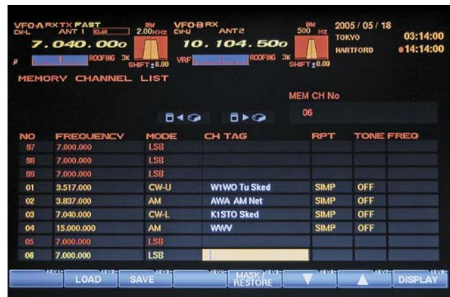
Figure 7—Memory channel annotation is possible, with data entered via a keyboard (not supplied).
