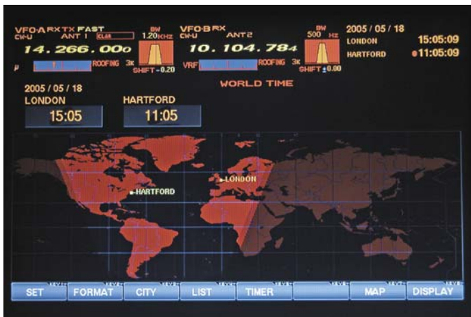
Figure 2—The TFT display showing key parameters, including the IF filter settings for both receivers, along with the top. This part of the display is common to most TFT displays. The bottom part of this display is the two-zone clock with approximation of areas of day and night.
