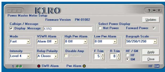
Figure 4—You can adjust a number of parameters and download firmware updates using the PowerMaster Lite software's METER SETUP screen.
