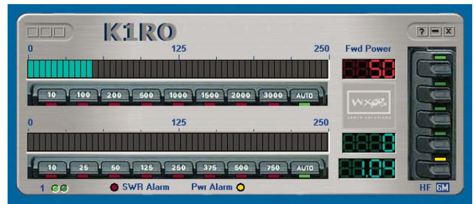
Figure 5—During normal operation the software displays both bar graphs and numerical readings for forward power (50 W) and reflected power (0 W) and a numerical reading for SWR (1.04:1). In this case, the forward power is displayed in red because the low power alarm has tripped.
