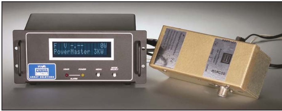
Figure 3—The PowerMaster display and directional coupler are packaged separately.
