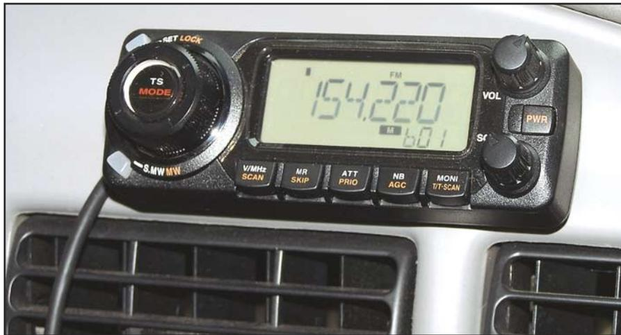
Figure 5 — The IC-R1500 control head installed on the dashboard of my car. What a great way to cruise the radio spectrum while cruising the highway!
