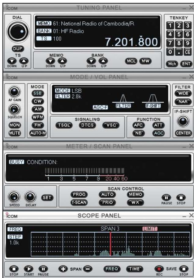
Figure 4 — The “component” screen that includes the band scope (bottom).
