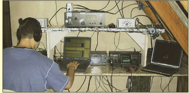
Figure A — Chris, KL9A, operating at PW5Q with the compact ACOM 1010 amp located between the run (left) and multiplier (right) stations. Aluminum foil on the shelf provided a temporary RF ground for the amp and filters.
