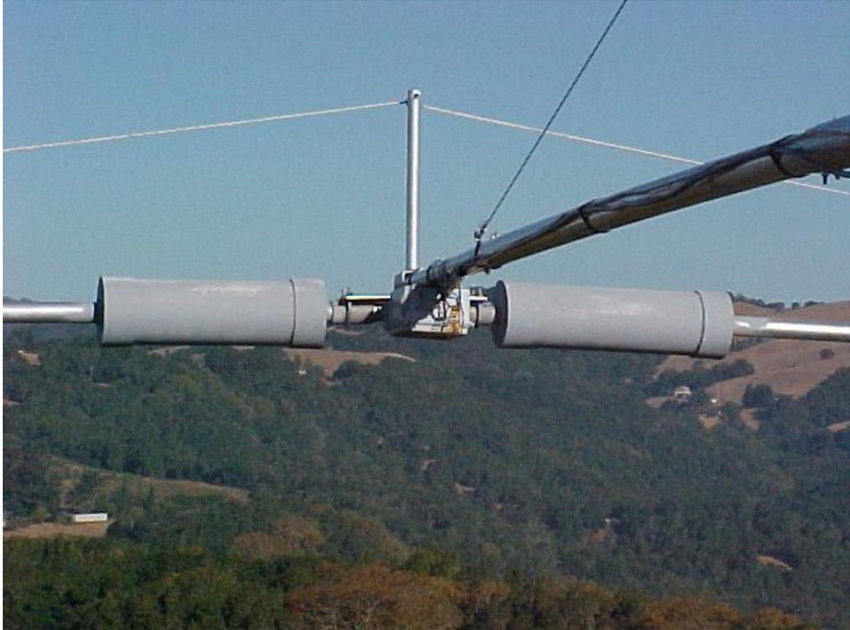
Center of driver element on Sigma 280S
