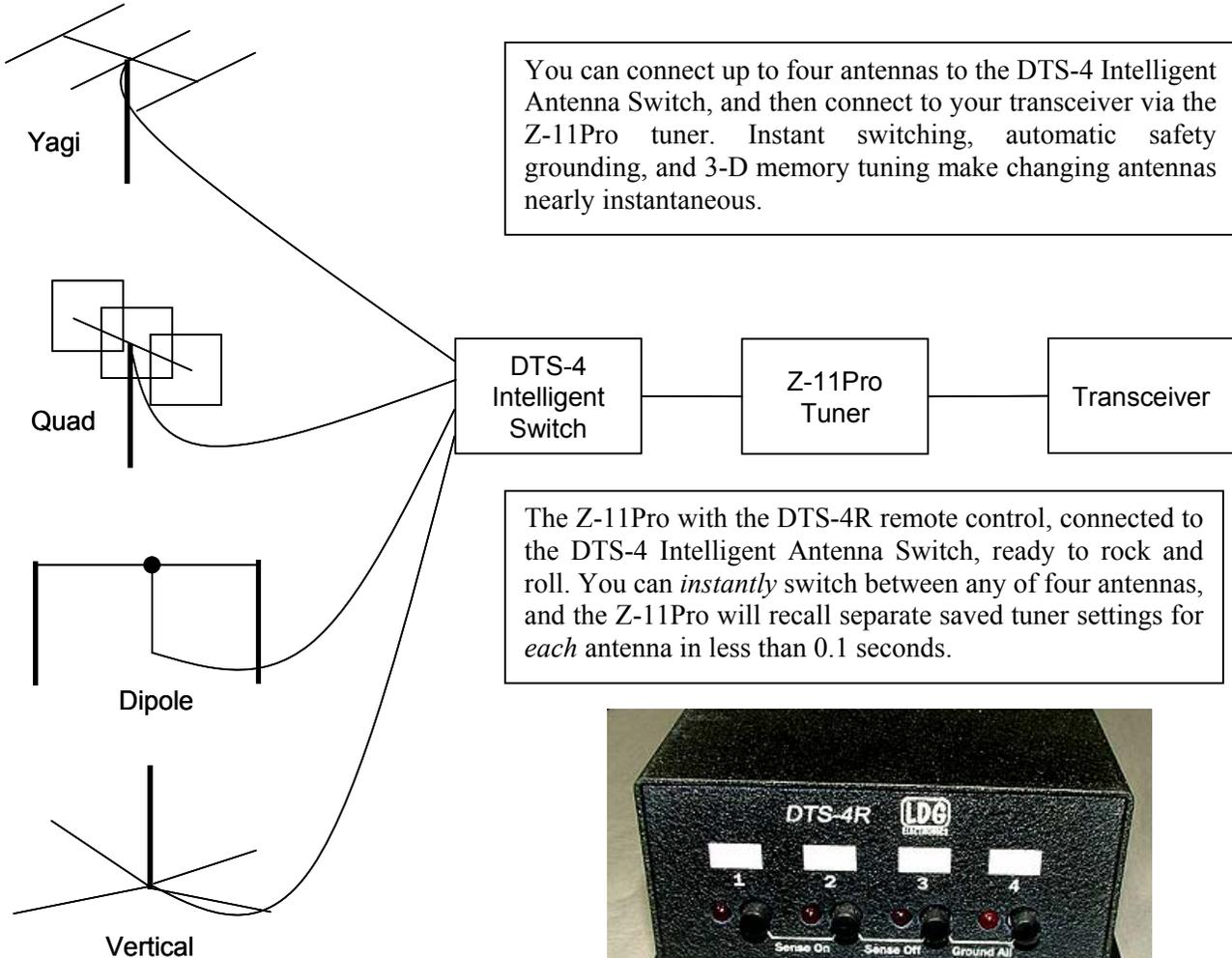
You can connect up to four antennas to the DTS-4 Intelligent Antenna Switch, and then connect to your transceiver via the Z-11Pro tuner. Instant switching, automatic safety grounding, and 3-D memory tuning make changing antennas nearly instantaneous.
